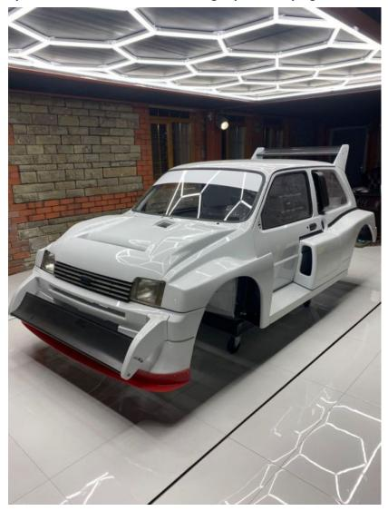
More details have emerged and, as promised, here is the update. The car will be powered by a 3.0 litre Audi engine from the Audi S4 with tuning to raise output from 350bhp to 450bhp driving through a Sadev six-speed sequential gearbox.
