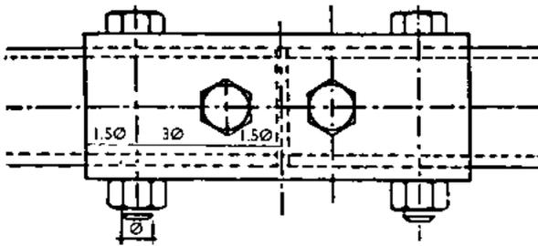
$\varnothing = 14\text{mm}$  (tube  $\geq 40\text{mm} < 50\text{mm}$  diam. ext.)
